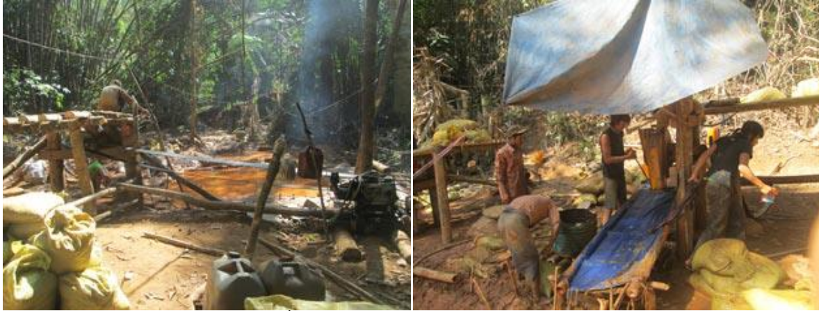
These photos were taken on January 5 th 2013 in Hsaw Htee Township, Nyaunglebin District and show gold miners who have been allowed to mine ore using a process known as cyanidation. This process involves placing crushed ore into piles where a cyanide solution is poured over it to dissolve the gold and allow it to “leach” out of the pile and also into the ground. This process risks contaminating the surrounding area and is heavily regulated by many nations. [Photos: KHRG]
