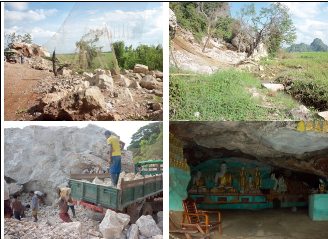
The above photos were taken on November 25 th 2013 in A--- village, Kyonedoe Township, Dooplaya District. The top-left photo shows a large net used to catch stones which may be propelled during the mining process. Nevertheless, larger stone projectiles may tear the net as can be seen in the photo. The top-right photo shows the farmers' irrigation canal that has been blocked by stones from the mining project. The bottom-left photo shows workers carrying stones and loading them on a truck in order to transport them to a rock crushing machine. The bottom-right photo shows the cave that local villagers use as a place of worship. Every year they celebrate traditional customs on this mountain, which is now under threat due to stone mining. [Photos: KHRG]
